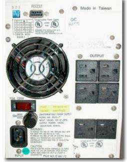
drops out of the circuit and the batteries keep the power steady and unchanged. When power is restored, the rectifier resumes carrying most of the load and begins charging the batteries, though the charging current may be limited to prevent the high-power rectifier from overheating the batteries and boiling off the electrolyte." Wikipedia
